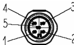
Standard Rexroth 12mm connection cable pin-out
