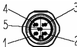
Standard Rexroth 12mm connection cable pin-out
