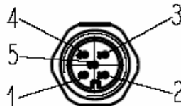
Standard Rexroth 12mm connection cable pin-out
